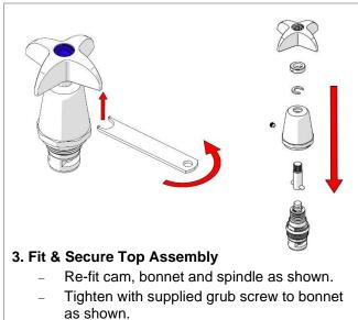
This is critical, failure to do so may result in damage and / or failure of the unit.
